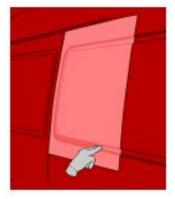
11. Check the application for remaining bubbles. If there still are small air bubbles to be seen, these can easily be removed. Just make a small puncture, heat it  $(40-50 \, ^{\circ}\text{C})$  and push the air out.
